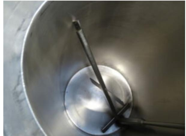
FONDOIR DOUBLE ENVELOPPE DESTINÉ AU MAINTIEN EN TEMPÉRATURE DE PRODUITS, AVEC CUVE CHAUFFÉE ÉLECTRIQUEMENT ET DISPOSITIF DE COULAGE MANUEL, ADAPTÉ AUX APPLICATIONS DE TRANSFERT OU DE DOSAGE DE PRODUITS FONDUS
