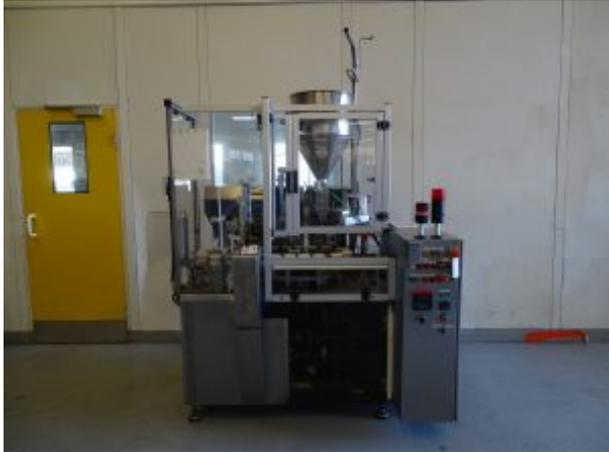
REPLISSEUSE DE TUBE AIR CHAUD
