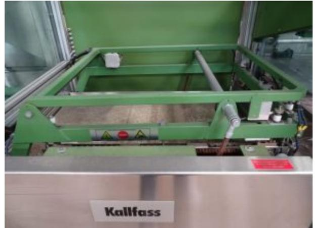
SOUDEUSE EN L AVEC FOUR DE RETRACTION
